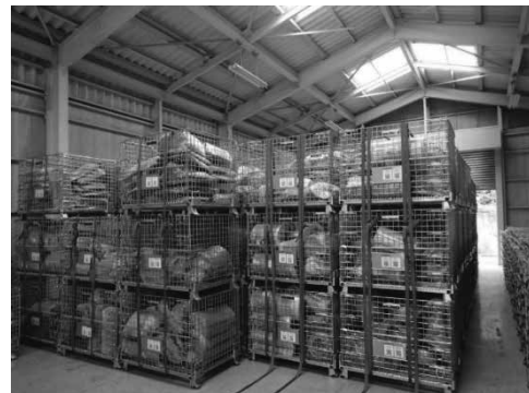
Fig.12 Storage of dismantled waste after Clearance measurement
