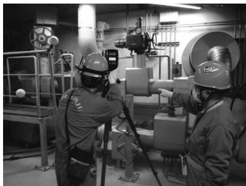
Fig.30 Work scene of point cloud data measurement with 3D laser scanner
